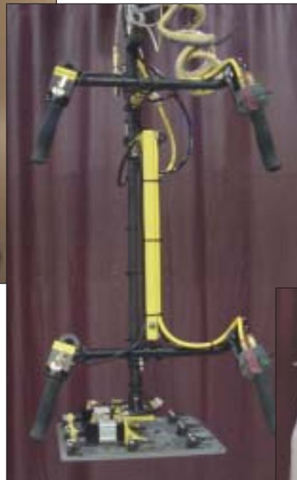
The spool handling device shown here used by a major pharmaceutical products manufacturer, has Dual Controls. The spools are stacked 3-high in a box and the Dual Controls enable the operator to pick up spools without bending.
