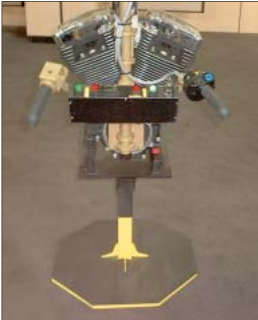
The engine handling device shown uses the unique features of the Intelift balancer. Features include: Auto Clamp, Interlock, Up control disable, weight sensing with automatic alarm, and keyed lock out.
