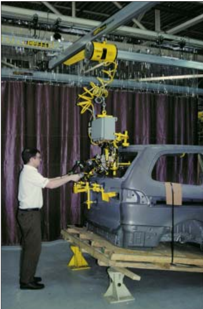
Vacuum end effector integrated with 4 Ingersoll-Rand D-Series nut runners shown installing a lift gate assembly.
