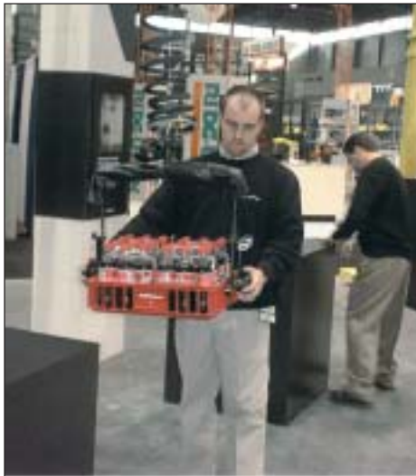
+ The warehouse handling device shown is known for its versatility. The device mimics the human motion of picking a part and placing it. The same device can be used to pick up parts such as totes, trays, boxes, and milk crates. The second picture shows the same device lifting a different part. The self balance feature allows the same device to pick up parts of different weights and sizes.
