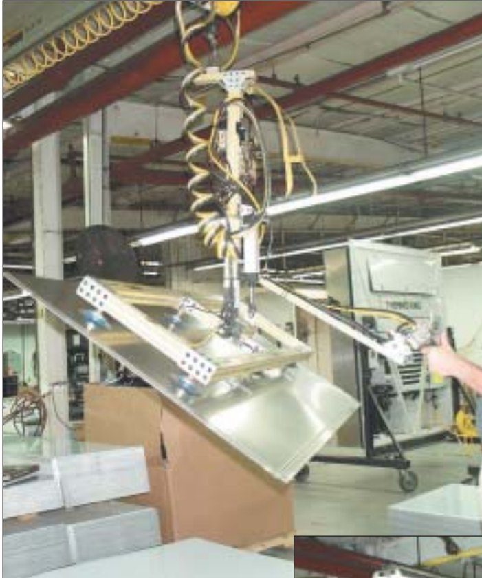
Ingersoll-Rand provided material handling solutions to Thermo King® in handling the back panel for a refrigeration unit. The handling device includes a Power Tilt feature.
