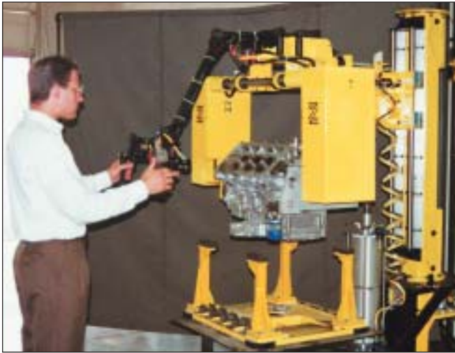
Air clamp handling device for engine rollover
